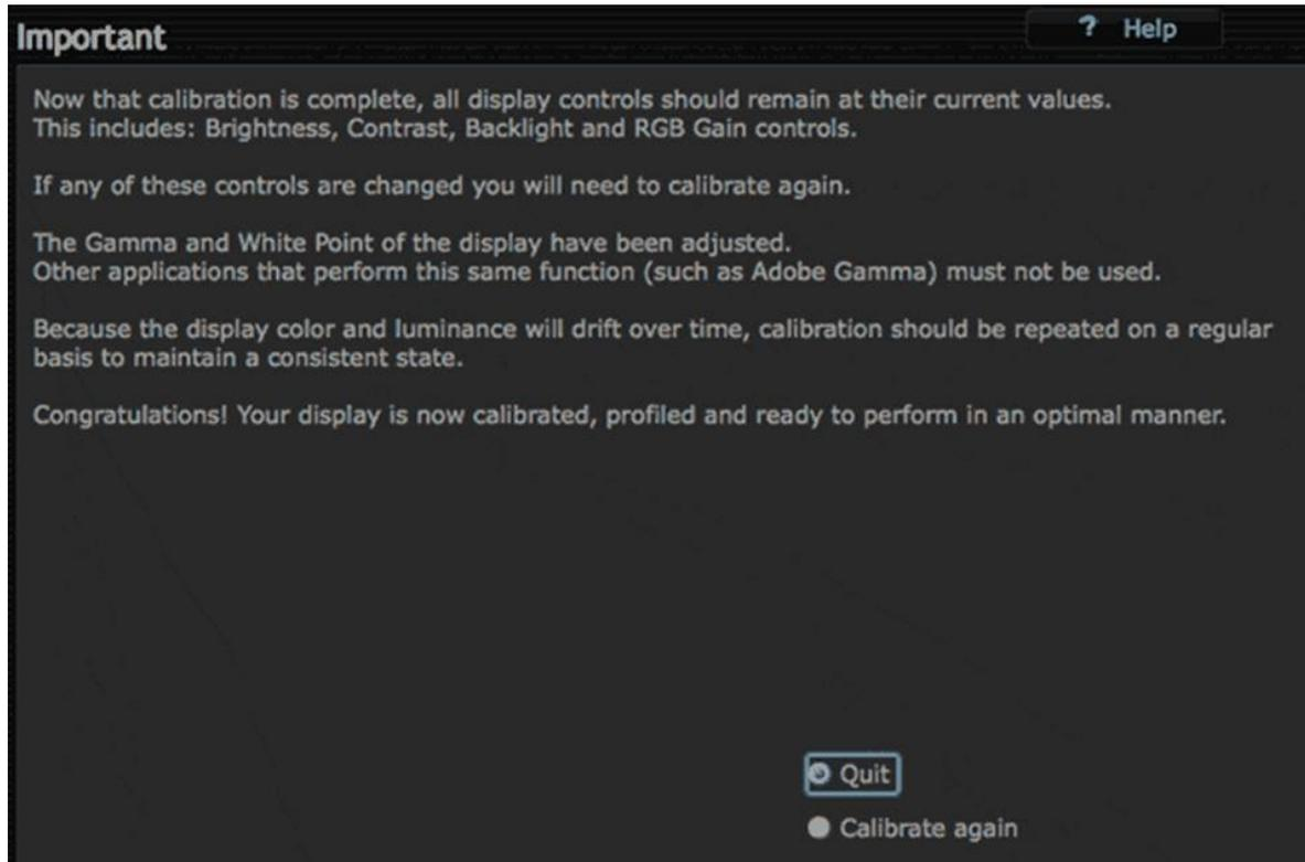
Over time the calibration can drift (see image above) so the process should be repeated regularly. The profile can be set to remind you of this and it is recommended this is used. The calibration should always be performed under the same conditions as far as practicable, same ambient light, time of day etc. to ensure meaningful results.
