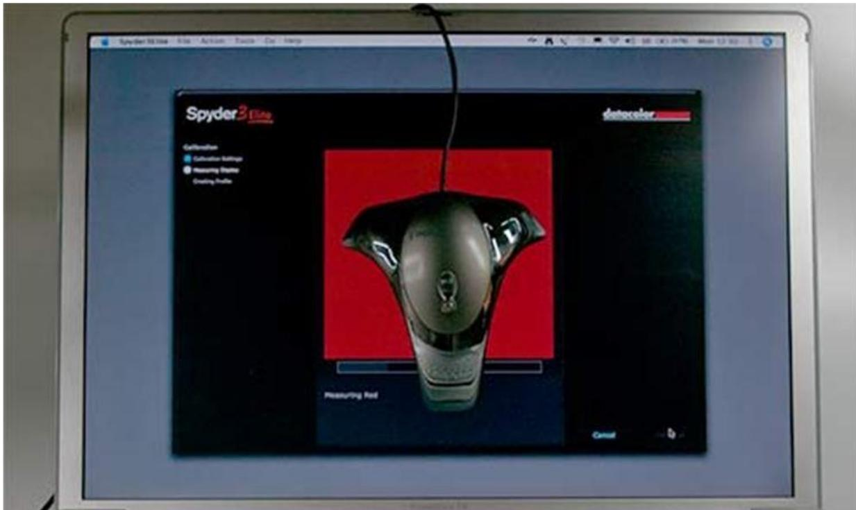
When the colors have finished being displayed the software writes a color profile for the monitor which is loaded into the video card and a test sheet of images is produced to show the before and after
