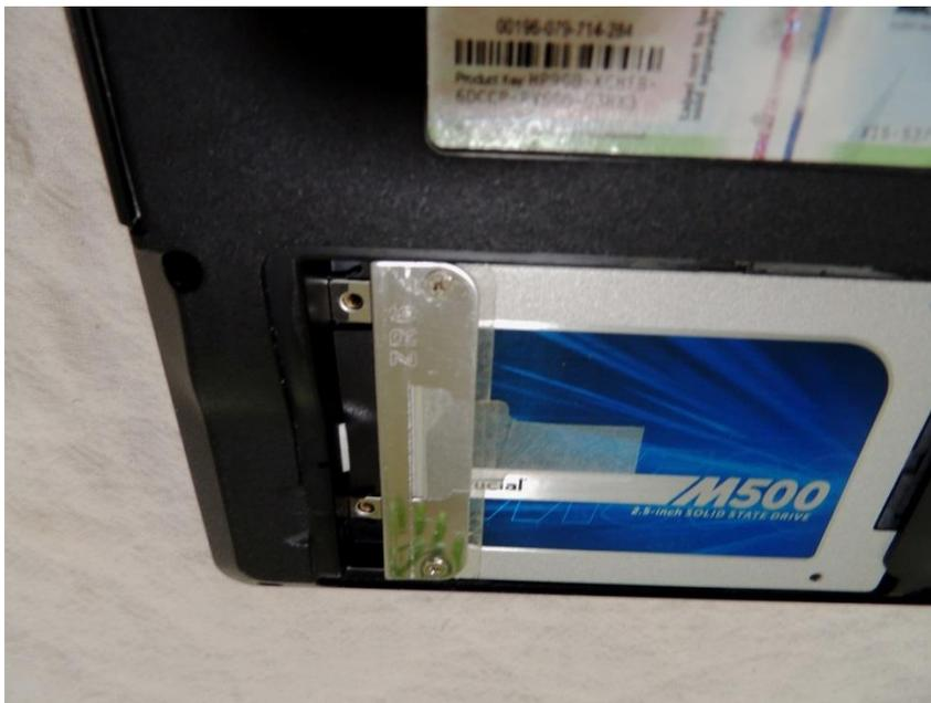
in place and the retaining plate fits into a slot between them and the drive base to keep the drive securely in place.
