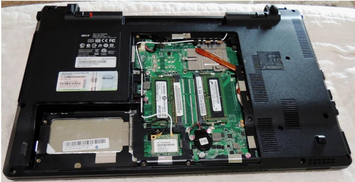
Take out the retaining plate and the drive can be slid out of the contact area towards the outer edge of the case. You can then remove the drive and set it aside, we will be using it again later.
