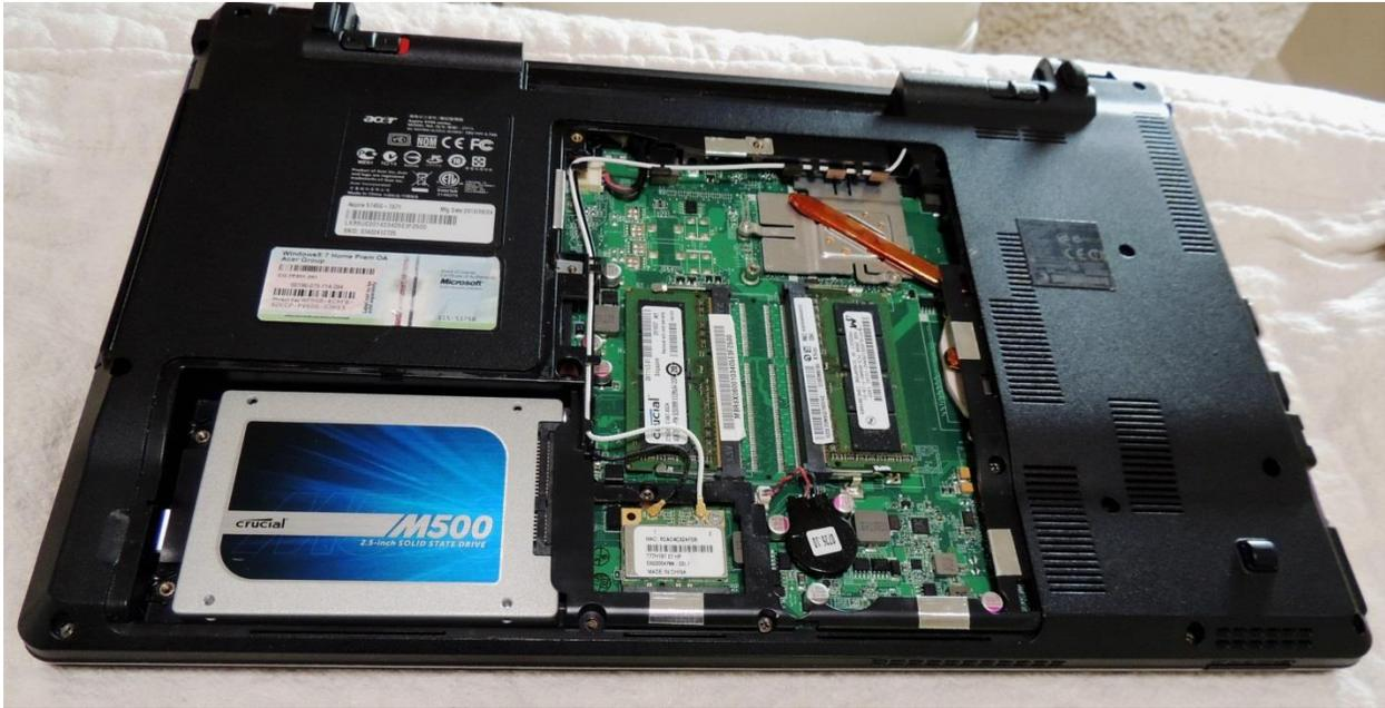
Here you can see the drive is in place and ready for securing.
